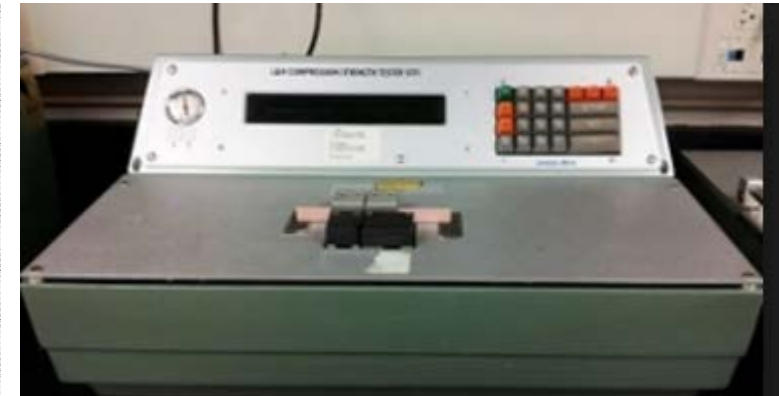
Figure 5. When the clamps move toward each other, the length decreases and the stress in the test piece increases until rupture occurs.
